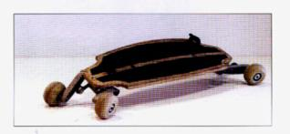
The steering geometry was perfected for this model. The ball-bearing polyurethane wheels stem from the running sections of escalators.
